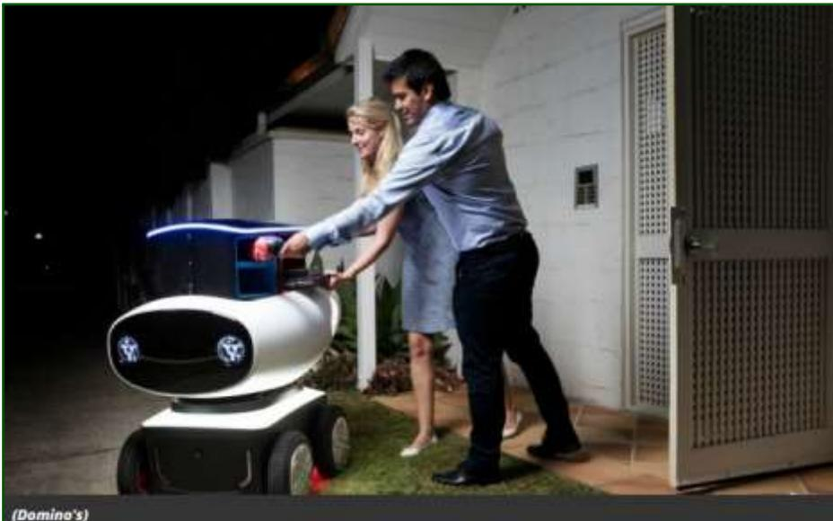
Domino's has unveiled its first pizza delivery robot in Australia. Called the **Domino's Robotic Unit**, or DRU for short, the machine is a military-grade prototype retrofitted for pizza delivery. It uses GPS to find customers' homes and carries pizzas and drinks in locked compartments that are opened by a mobile phone code sent to the customers. DRU also talks.
